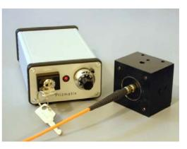
chopping mode operation with preset frequency and duty cycle.
