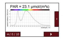
Display of PAR and the spectral power distribution
