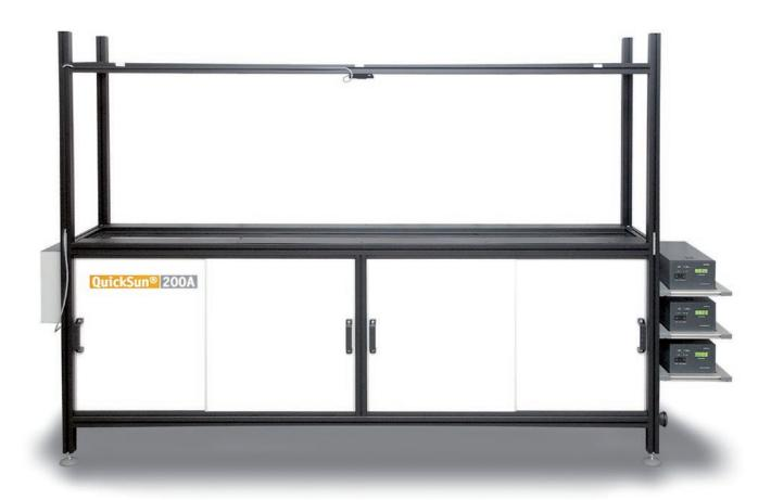
QuickSun 200A String Simulator is a new cost-efficient tool for improving yield and maximizing module power. It provides a full I-V curve for strings as large as 20 x 200 cm<sup>2</sup> with a maximal rate of 360 measurements per hour. All the essential performance parameters are included, with the possibility for series resistance evaluation according to the IEC 60891 standard.
