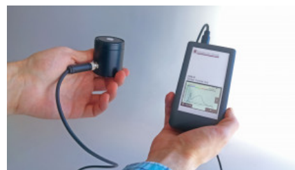
Use of CSS-45 as a handheld instrument by combining it with the control unit CSS-D
