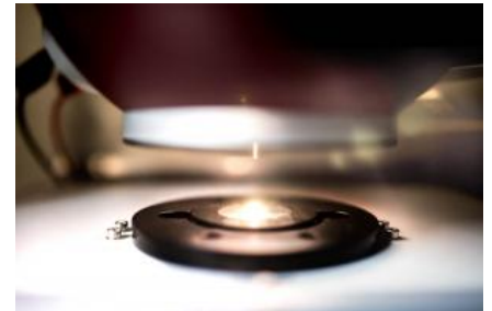
The integrating sphere moves motor driven in the measurement position
