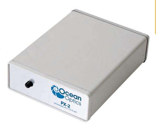
In the Single mode of PX-2 operation, a single flash occurs during each integration period. The flash rate is modified by changing the integration period. Because it produces a pulsed signal, the PX-2 is less likely to contribute to solarization in optical fiber assemblies, which can occur when fibers are illuminated with signal <260 nm.
