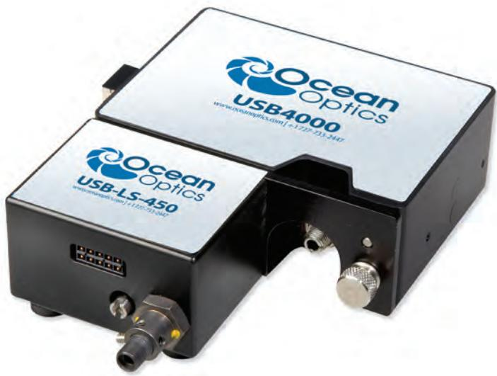
The USB4000-FL, USB4000-FL-450 and USB4000-FL-395 Spectrometers are preconfigured for fluorescence measurements from 360-1100 nm. Each spectrometer comes with a 200  $\mu\text{m}$  slit and detector collection lens for increased light throughput and features plug-and-play operation, a high-performance 3648-element CCD-array detector and fast USB 2.0 connectivity.
