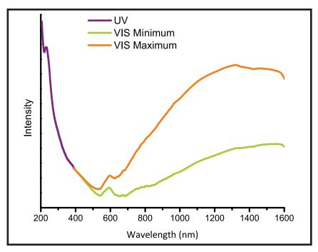
The UV-Vis-NIR output spectrum of the DH-mini Light Source from 200 - 1600 nm. The output intensity of the tungsten source is adjustable between the minimum shown in green and the maximum shown in orange. The tungsten source emission range extends to 2500 nm (data not shown).
